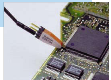
The HP Wedge provides dependable, trouble-free connection to fine-pitch ICs.
