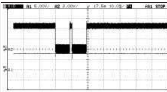
Figure 3: Once the glitch was identified, zooming in to a faster time base setting provided the necessary details.
